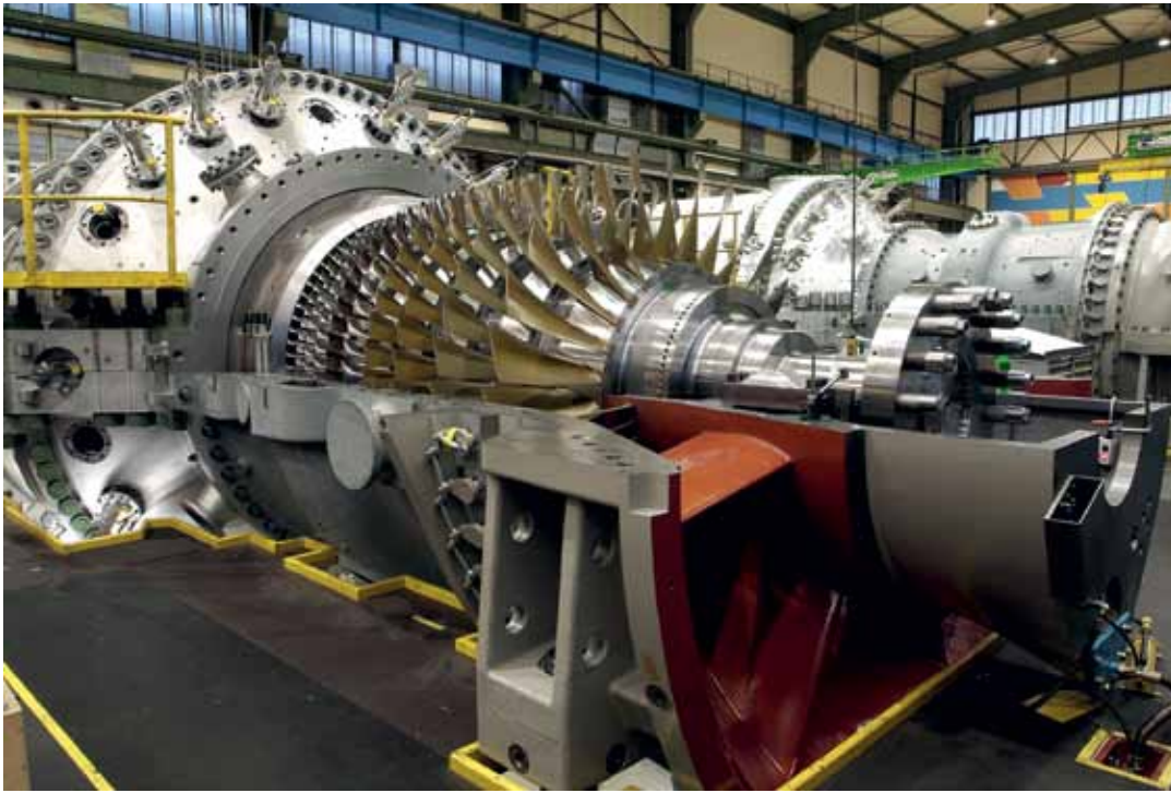
Figure 2: Large power plant gas turbines in production; construction time several months; the Technical Writing department delivers the documentation before the gas turbine arrives at its destination. © Siemens Energy
